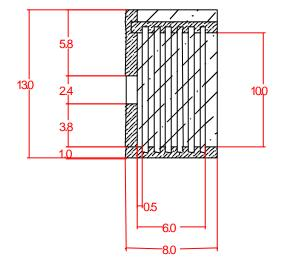
Figure 2: Plexiglas box containing the samples
