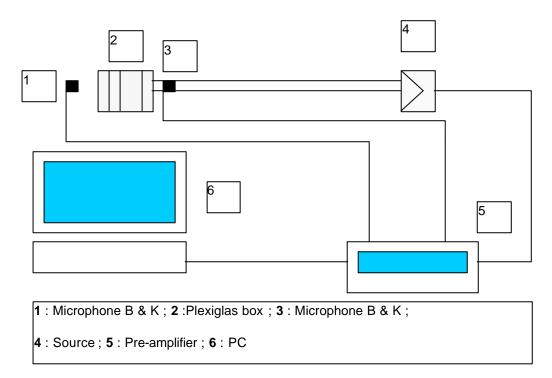
Figure 1 : Acquisition chain of the experimental set-up
