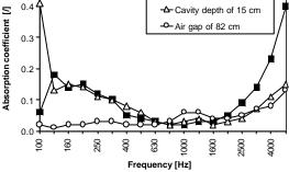
Figure 8 – Absorption coefficients for configurations with plates laid on rectangular frame and different cavity depths
