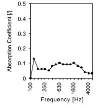
Figure 10: Absorption coefficients of the sample of suspended ceiling tested in the reverberation room
