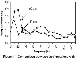
Figure 4 – Comparison between configurations with different studs pitch (60 and 40 cm)
