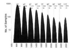
Exemple of Jitter histogram corresponding to each pit lenghts of a CD-R. Some confusion are possibles in recognising 3T/4T to 5T/6T.
