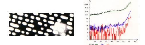
Every obstacle (on optical disc here) will improve error rate. On the right example, error correction processing can't compensate such an increasing level at the end of the disc.
