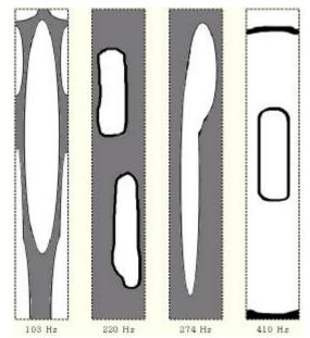
Fig. . Chladni patterns of the top plate
