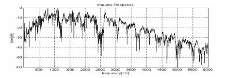
Fig. . Impulse response of the top plate only
