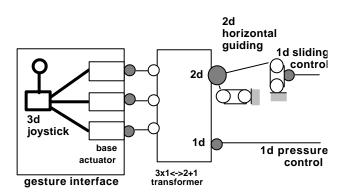
Figure 2. The 3d bowing force feedback joystick and its coupling to the bow simulation.
