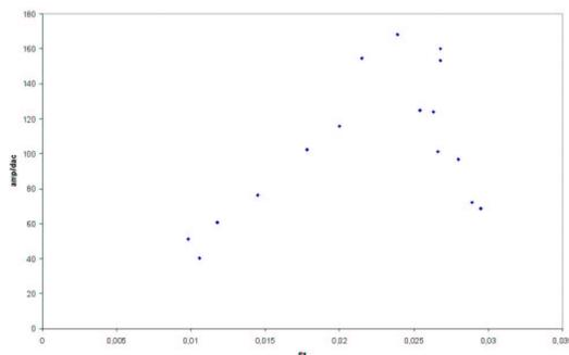
Figure 5: Influence of Strouhal number over adimensional amplitude, for a constant Reynolds number ( $Re = 2600$ ).
