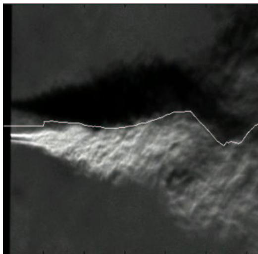
Figure 2: Center line detection by image filtering
