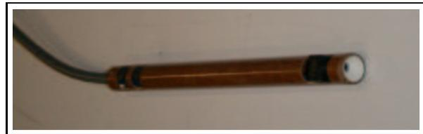
Figure 6: Synthetic flute with sensors.
