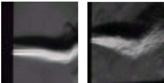
Figure 3: Jet under acoustic excitation by loudspeakers. Left: Laminar jet,  $Re = 600$ ; Right: turbulent jet,  $Re = 4000$
