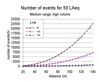
or the medium range, high volume situation a somewhat higher level is required then in the typical urban situation. An Lwa of 95 dB(A) permits traffic up to 2000 vehicles per hour at 50 m distance, or 10000 /hr at 100 m distance. This last figure corresponds to the carrying capacity of a 6 lane motorway.
