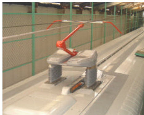
Fig. 1 Example of Low noise pantograph (Type PS207 of JR-East )
