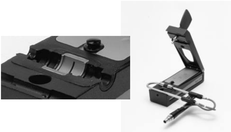
Figure 2. Photographs of the final calibrator. The probe is a \frac{1}{2} probe with a 12 mm spacer. The slit with the sound source is seen in the middle of the coupler cavity.
