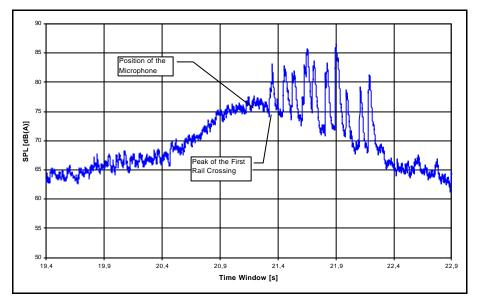
Fig. 2: Pass by level of a car - 46 km/h (VW-Golf)
