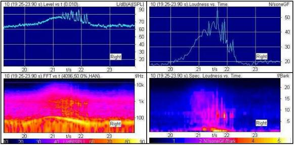
Fig. 3: Acoustical behaviour of a rail crossing by a car
