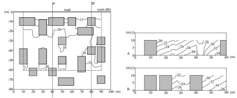
Fig. 9. Examples of noise distribution as an application of equation (1)
