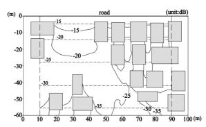
Fig. 10. Example of noise distribution as a comparison between ASJ Model 1998 and equation (1)
