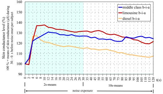
Fig. 5.- Skin conductance level for the pass-by noises of the three different cars at the b-i-a situation.
