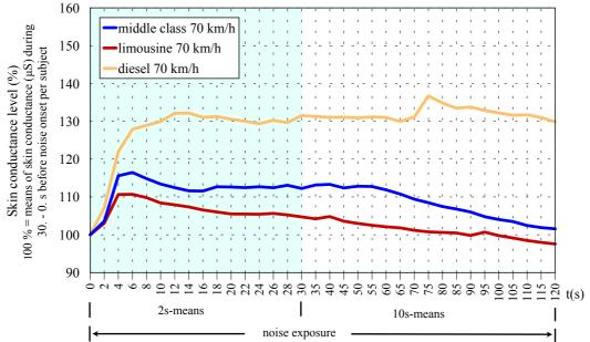
Fig. 2.- Reaction of skin conductance level to pass-by noises of 3 different cars at 70 km/h constant speed.
