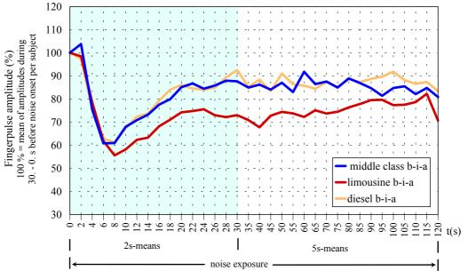
Fig. 4.- Reaction of fingerpulse amplitude to pass-by noises of 3 different cars at the brake-idleacceleration situation.
