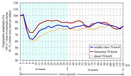
Fig. 1.- Reaction of fingerpulse amplitude to pass-by noises of 3 different cars at 70 km/h constant speed.
