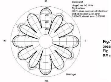
**Fig.1:** Directivity pattern of the sound pressure level for the sphere shown in Fig. 2, f = 100 Hz; solid line = iterative BE solution, circles = analytical solution.
