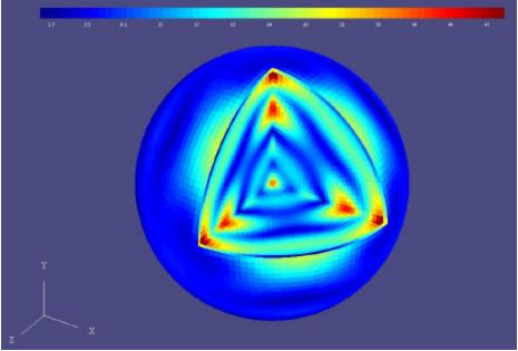
**Fig. 5:** Relative, local error of order n = 0, m = 0 on the surface of the cat's-eye at f = 500 Hz.
