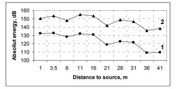
**Fig. 3.** Change in the absolute energy of direct sound of unfiltered signal and of the first reflections depending on the distance to the sound source and the length of pulse measured. 1 - only direct sound, from 0 to 0.4 ms; 2 - from 0 to 50 ms.
