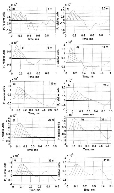
**Fig. 2.** Dependence of the amplitude and form of direct sound of an unfiltered signal upon the distance to the sound source. a), b), c), d), e), f), g), h), l), j) – distance from the microphone to the sound source is equal to 1, 3.5, 6, 11, 16, 21, 26, 31, 36 and 41 m respectively.
