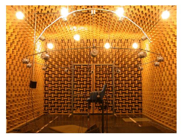
Fig. 3: Experimental setup in anechoic room
