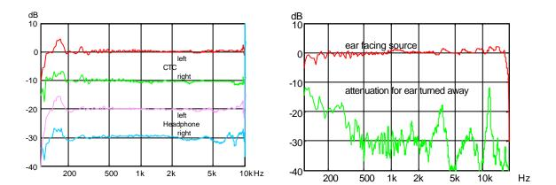
Fig. 6: Deviation of frequency response in comparison to loudspeaker reproduction.
