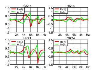
Fig. 1: Additional acoustical load on the ear of four headphones under test
