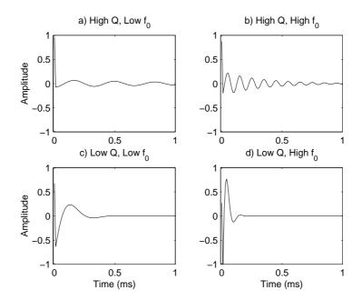
Figure 3 Impulse responses of the four second order all-pass sections shown in Figure 2.
