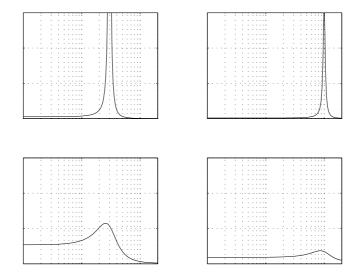
**Figure 2** The group delay of a second order all-pass section is shown with the following properties: a) High Q, Low  $f_0$ , b) High Q, High  $f_0$ , c) Low Q, Low  $f_0$ , and d) Low Q, High  $f_0$ , where High Q = 10, Low Q = 1, Low  $f_0$  = 3 kHz and High  $f_0$  = 10 kHz.
