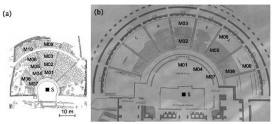
Figure 2. Sound source (S) and receivers (M01-M10). (a) Delphi; (b) Taormina.
