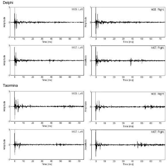
Figure 3. Binaural impulse responses as typical examples of the measurements.
