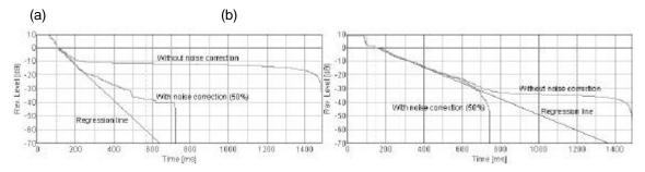
Figure 4. Decay curves for reverberation obtained by Schroeder's method as typical examples of the measurements. (a) Delphi (at M05) (b) Taormina (at M07).
