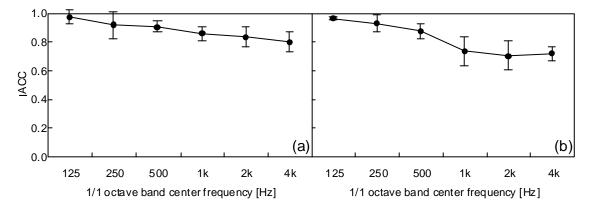
Figure 6. Results for IACC. Average value of 10 receiver positions and standard deviations are indicated. (a) Delphi; (b) Taormina.
