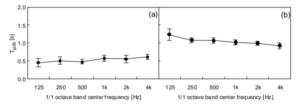
Figure 5. Results for  $T_{sub}$ . Average value of 10 receiver positions and standard deviations are indicated. (a) Delphi; (b) Taormina.
