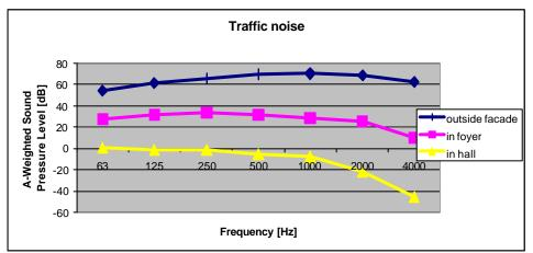
Figure 20: Estimated noise levels in the foyer and main auditorium with the application of the laminated glass.
