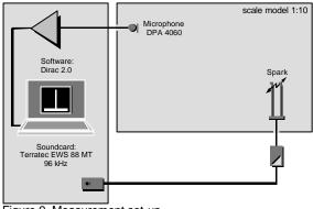
Figure 9. Measurement set-up.
