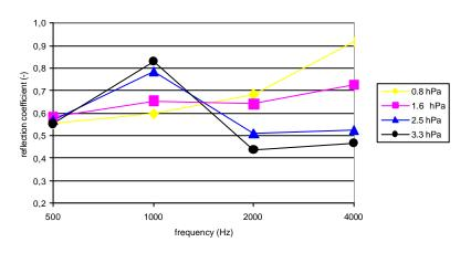
Figure 15: Reflection coefficients of canopy under different pressure conditions.
