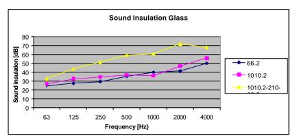
Figure 19: Sound insulation of laminated glass, measured in the acoustics laboratory of the Eindhoven University of Technology.
