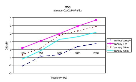
Figure 14: Calculated C<sub>50</sub> for different canopy positions.
