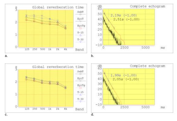
Figure 5: Estimated reverberation time and echogram in case of non-diffuse (a and b) lateral wall finishing and diffuse (c and d) lateral wall finishing.
