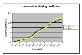
Figure 17: Measured scattering coefficient in a scale model on a scale sample of corrugated glass and RPG QRD flutterfree diffusor.
