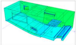
b. Geometric model with maximum detail corrugated glass as one surface
