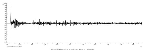
C:\portolS1R2 canopy 10 m spark.wav - Pressure - Allpass Hz Figure 11: Impulse response source position 1, receiver position 2., canopy height 10 m
