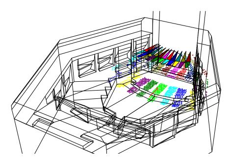
Fig. 2 Coverage by reflectors before alterations.
