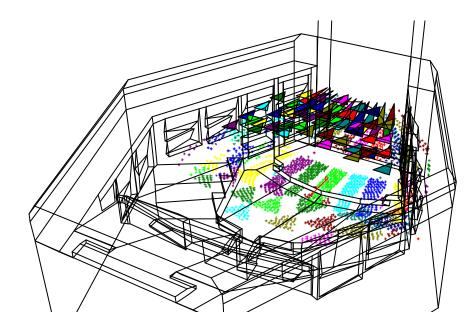
Fig. 3 Coverage by reflectors after alterations.
