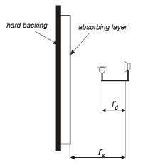
Figure 1: The measurement set up.
