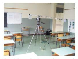
Figure 5: Pre-modification examination – in situ control of the acoustic performances.
