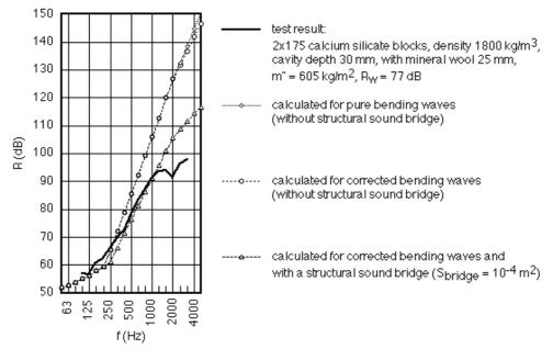
Fig. 2: Measured and calculated sound reductions indeces for a heavy double wall
