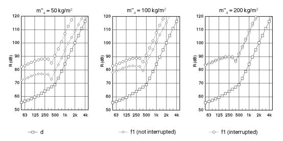
**Fig. 4:** Sound reduction index per element for different surface mass of the outer leaf (separating element: 2 x 100 mm concrete 2300 kg/m<sup>2</sup>, flanking element: 100 mm aerated concrete 700 kg/m<sup>2</sup>), without and with interruption the outer leaf with surface mass m<sup>\*</sup><sub>4</sub>).
