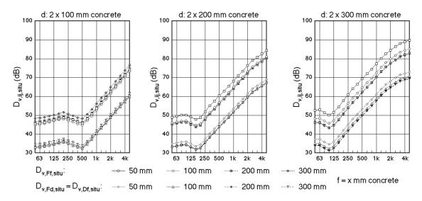
Fig. 3: Direction-averaged junction velocity level differences for flanking paths Ff, Fd and Df for 3 types of separating heavy double walls (d) and for 4 types of flanking elements (f) each.
