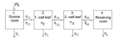
Fig. 1: SEA-systems with energy flows for modelling a double wall
