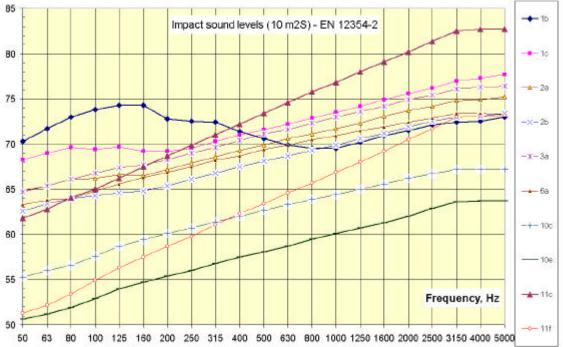
Figure 1. Impact sound pressure levels of the cases given in Table 1. The variation in level and shape of the curves indicates that the performance of a specific flooring will depend on the slab and boundary conditions.
