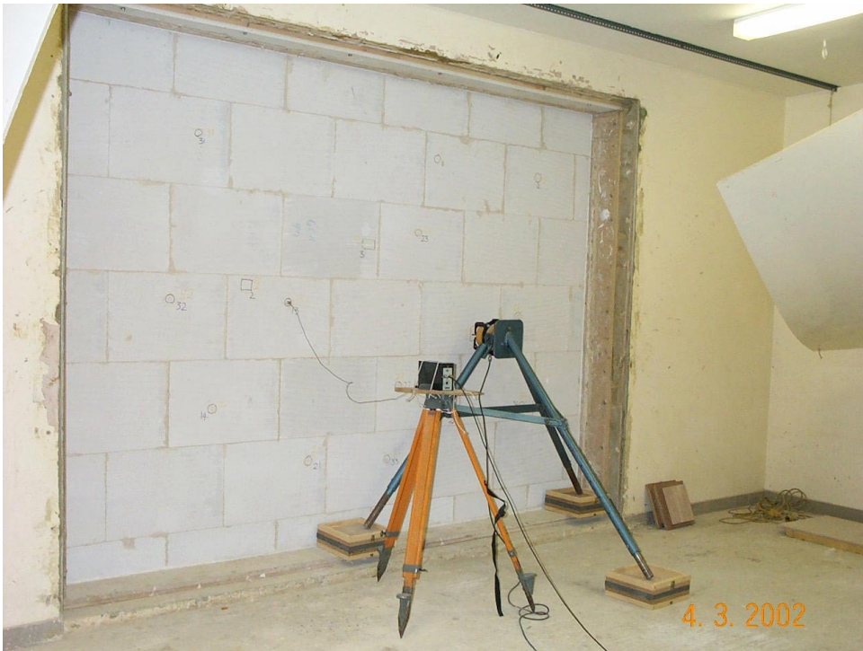
Figure 1 : MLS vibration method. Charge amplifier, accelerometer and electrodynamic shaker in the transmission suite.
