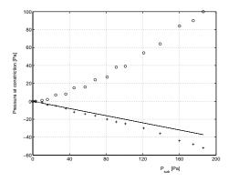
Fig. 2.- Pressure evolution at constriction, *hc*=1.63mm as a function of *Psub* (+) upper wall (o) lower wall.(+) experimental points (straight line) simple theory assuming a fixed separation point.
