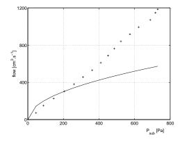
Fig. 5.- Flow evolution *Pgd* as a function of *Psub* for the latex tongue and a constriction height of *hc*=0.4mm.
