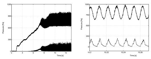
Fig. 6.- Self-sustained oscillations obtained with the experimental setup Upper curve :Psub, lower curve *Pgd*.
