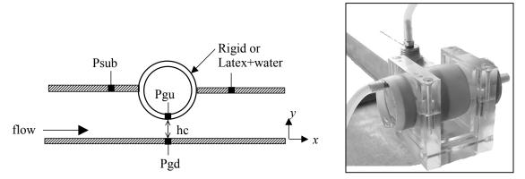
Fig. 1.- Schematic view and photography of the experimental setup used to study airflow/tongue interaction.
