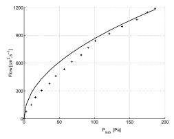
Fig. 4.- Flow evolution as a function of Psub. Rigid tongue, constriction height hc=1,63mm (+) experimental points (**straight line**) simple theory assuming a fixed separation point (see text).
