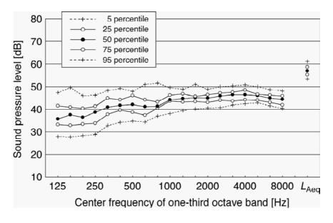
Fig. 5 Graphical data showing domestic sound frequency characteristics. (A sound of washing dishes.)
