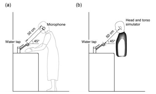
Fig. 4 A setting of recording apparatus and materials. (a) A microphone, (b) a head and torso simulator. (Recording of a sound of washing dishes.)
