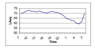
Figure 1. Acoustic profile of a street confirming the results obtained
