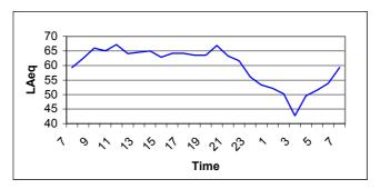
Figure 2. Acoustic profile of a street with a drop of 10 dBA between  $L_{\!\scriptscriptstyle d}$  and  $L_{\!\scriptscriptstyle n}.$
