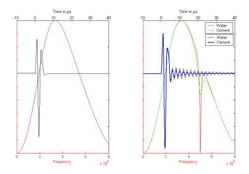
Figure 3: Modeled time and frequency response of the transducer after reflection on a single interface (left), and after reflection on a steel plate backed by water or cement (right).
