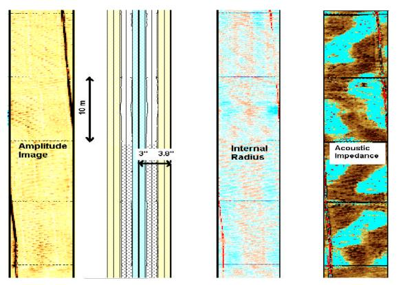
Figure 4 : Cement behind casing evaluation (see text for explanations).
