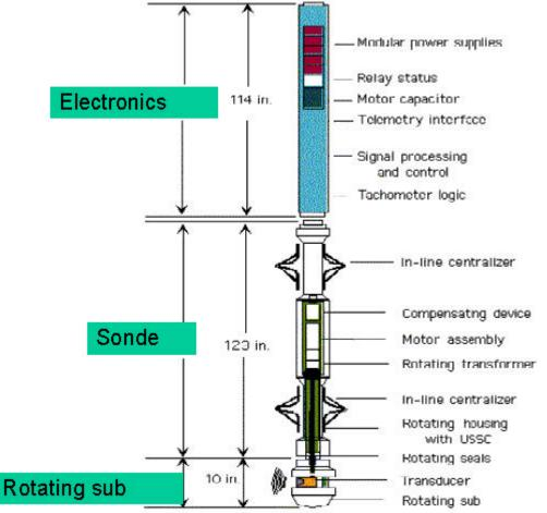
Figure 1: Schematic of the ultrasonic sonde.
