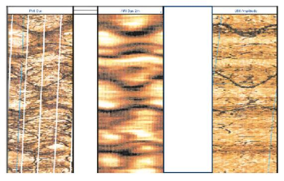
Figure 2: Example of ultrasonic amplitude image (right track) compared with high and low resolution resistivity images (left and center track). Vertical distance 13m.
