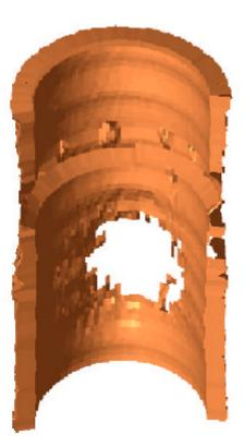
Figure 5: 3D images of short pipe sections from ultrasonic measurement of inner radius and thickness.
