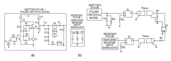
Figure 1. Emitting and Receiving models in PSPICE diagram for the electrical stages a) Pulser circuital model b) Simplified receiver input impedance
