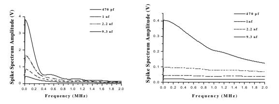
Figure 5. Spike frequency spectra amplitudes for different values of Cd and light damping conditions (Rd = 470 Ohm). Figure
