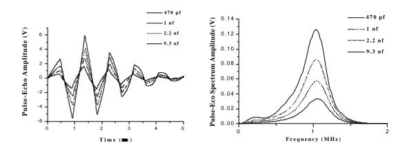
Figure 7. Pulse-Echo temporal responses for different Cd values and light damping conditions (Rd = 470 Ohm).
