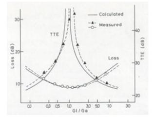
Fig.4. Measured data and calculated curves of insertion loss and triple transit echo.
