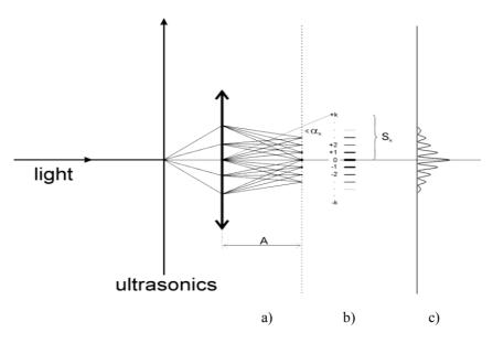
Fig 3. Raman-Nath model of the ultrasonic light diffraction for normal incidence: a)interaction and diffraction scheme, b) diffraction pattern at the focus plane of a lense, c) light intensity distribution in diffraction pattern for several orders.
