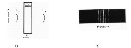
Fig 1. Original Debye and Sears' optical arrangement for the ultrasonic light diffraction (a) and the original spectrum of multiple diffraction orders (b) for 5.7 MHz after [2].
