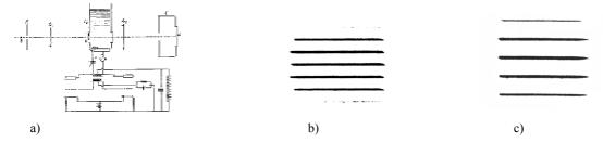
Fig 2. Original Lucas and Biquard experimental arrangement for the ultrasonic light diffraction (a) and their original spectra of multiple diffraction orders for 30.3 in the water (b) and 30.3 MHz in petroleum ether (c).
