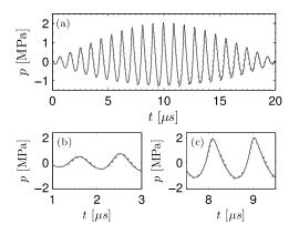
Fig. 3. Experimental (dashed line) and KZK simulated (continuous line) waveform measured at The input voltage in the experiment was 228 Vpp and the initial pressure in simulation was 105 kPa, chosen to produce equal pressure at the focus. (a) Complete half-period of the AM signal, where linear and nonlinear propagation coexist at different times. (b) Initial small-amplitude oscillations and (c) central oscillations of the AM signal, where strong nonlinearities are produced.
