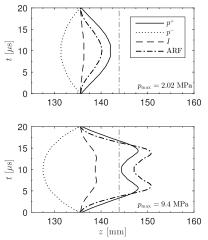
Fig. 7. On-axis focal displacements for a 25 kHz-AM beam in liver. Peak pressure (solid line), rarefaction minimum (dashed line), intensity (dotted line). The vertical dashed line shows the geometrical focus. (a) Weakly nonlinear scenario, (b) strongly nonlinear scenario.
