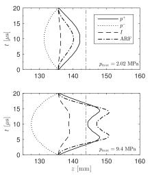
Fig. 5. On-axis dynamic focal displacements in water for a 25 kHz AM signal. Top: moderate nonlinear regime. Bottom: strong nonlinear regime. Peak pressure (solid line), rarefaction minimum (dashed line), intensity (dotted line) and ARF (dasheddotted line). The vertical dashed line shows the geometric focus. (a) Weakly nonlinearity scenario, (b) strongly nonlinear scenario.
