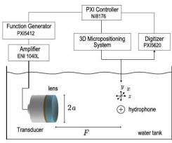
Fig. 1. Scheme of the experimental set-up for the pressure measurement in water.
