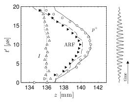
Fig. 4. On-axis simulated (lines) and experimental (markers) of the peak pressure (white circles), maximum intensity (white triangles) and maximum ARF (Black triangles) locations obtained for each period of the AM-carrier component. t0 is the dimensionless retarded time, where the time delay due to wave propagation distance has been eliminated.
