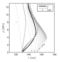
Fig. 6. (a) On-axis maximum pressure, p., intensity, I., and ARF location obtained from the KZK simulation of the ultrasonic beam in tissue. Numbered gray lines represent the on-axis maximum pressure location of each harmonic. (b) Axial pressure profiles for increasing source amplitude, p0 (increasing from gray to black). The thick black line shows the peak pressure location, p.. The vertical dashed dotted line marks the geometrical focal.
