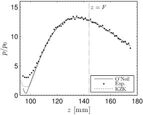
Fig. 2. On-axis maximum pressure distribution for small amplitude wave propagation obtained by experimental data (dots), O'Neill solution (solid line) and KZK numerical solution (dotted line). The vertical dashed-dotted line shows the position of the geometric focus.
