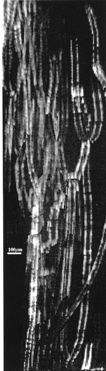
Figure 5: Multiple agglomerations (Chain reaction), 8.1 \mu\text{m} microspheres, frequency 800 Hz, acoustic velocity 0.45 m/s
