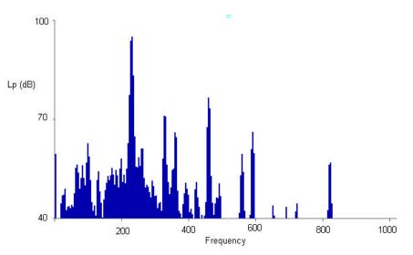
Figure 4. Noise spectrum of the electric motor.
