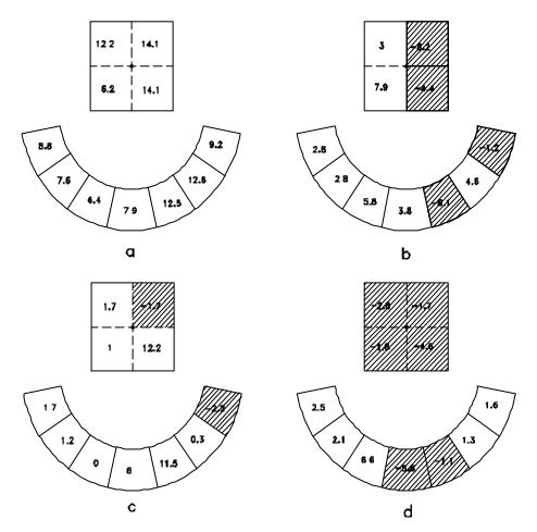
Figure 3. Attenuation levels in the window and outside the window, at the frequencies of a) 280 Hz, b) 550 Hz, c) 1100 Hz and d) 2200 Hz.
