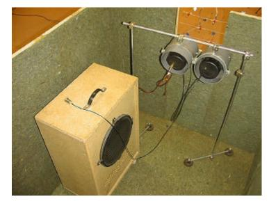
Figure 2. Location of the sound sources and control microphones.
