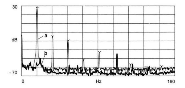
Fig. 3 Spectrum of the force transmitted to the foundation with (b) and without (a) active vibration isolation.
