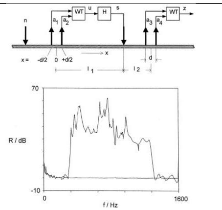
Fig. 4 Principal arrangement and transmission loss of an active reflector
