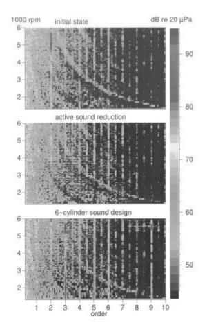
Fig. 7 Order spectra of the sound level at the drivers position during a slow run-up on the road
