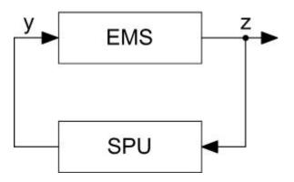
Fig. 2 Scheme to illustrate the control of target quantities **z** of an electromechanical system EMS by suitably driving the control inputs of EMS.
