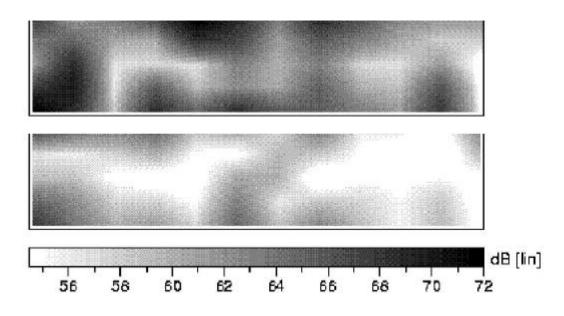
Fig. 5 Spatial distribution of the sound pressure level in the compartment of an ICE high speed coach with (below) and without (above) active control
