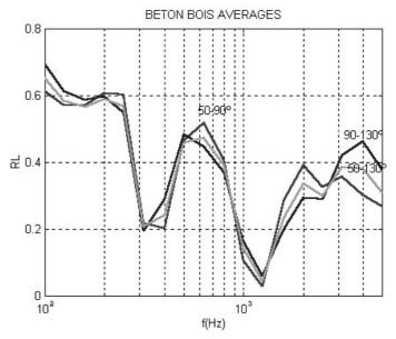
Figure 3. Averaged Reflection Loss curves on Beton Bois for 50-90°, 90-130°, and 50-130°.
