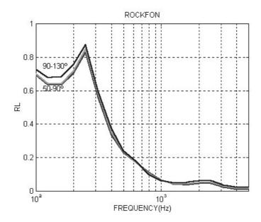
Figure 2. Averaged Reflection Loss curves on Rockfon for  $50^{\circ}-90^{\circ}$ ,  $90^{\circ}-130^{\circ}$ , and  $50^{\circ}-130^{\circ}$
