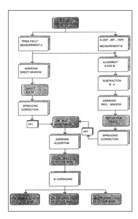
Figure 1. The MLS method with signal subtraction technique
