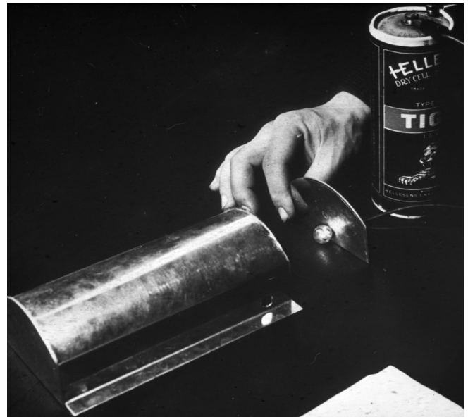
Fig. 3. Optical model of a hall with a concave ceiling. The energy distribution on the floor can be studied on a photographic plate.
