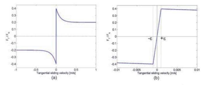
Figure 2 – Evolution of the friction coefficient with the contact relative tangential velocity ( $\mu_{\infty} = 0.2$ ,  $\mu_s = 0.4$ , C = 10): (a) For  $-1 < \dot{\tilde{y}}_t < 1$ ; (b) For  $-0.01 < \dot{\tilde{y}}_t < 0.01$
