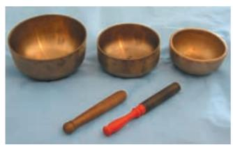
Figure 1 – Picture of three singing bowls and pujas: Bowl 1 ( $\phi$ =180 mm); Bowl 2 ( $\phi$ =152 mm); Bowl 3 ( $\phi$ =140 mm).
