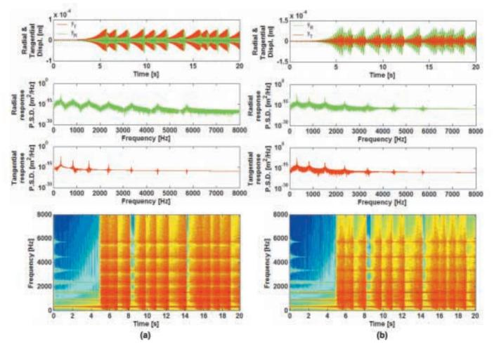
Figure 5 – Time-histories, spectra and spectrograms of the dynamical response of Bowl 2 to friction excitation when  $F_N = 1 N$ ,  $V_T = 0.5 m/s$ : (a) at the bowl/puja travelling contact point; (b) at a fixed point of the bowl's rim
