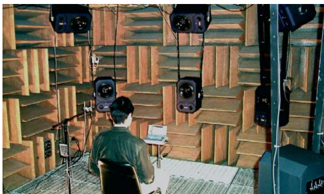
Figure 17. Eight-channel sound field simulation system in anechoic room.
