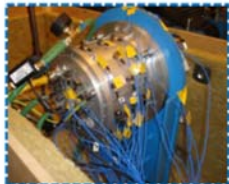
Fig. 7: Test rig with a SR drive system coupled to a two-pole induction motor
