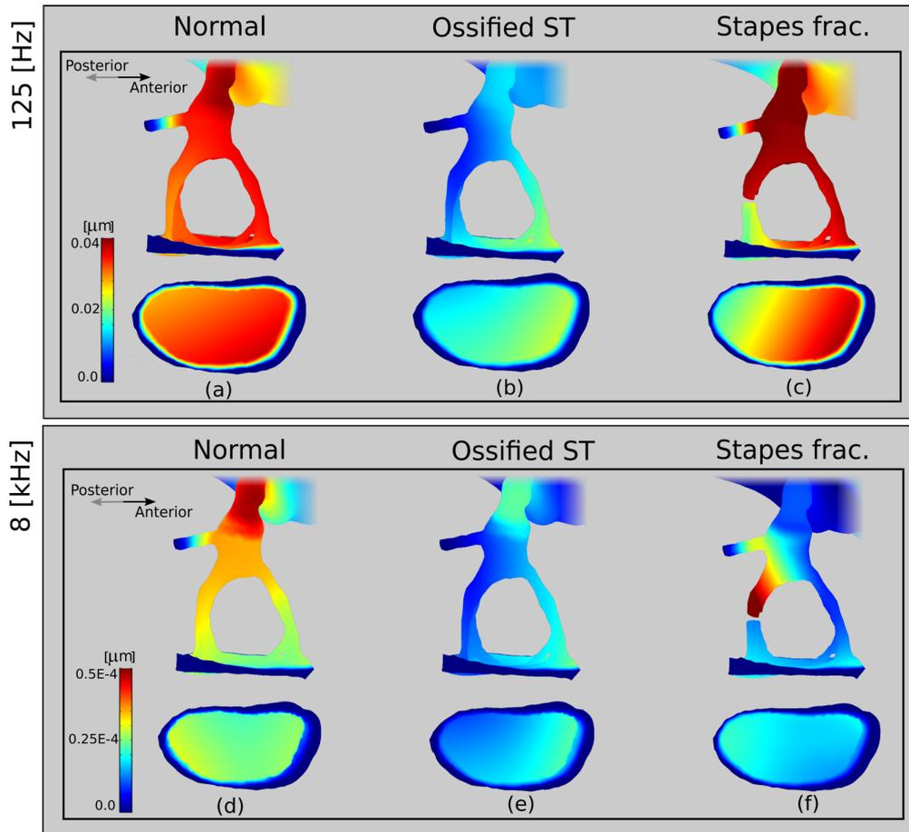
Figure 5: Total displacement  $u$  of the stapes (inferior view) and its footplate (medial view) under normal and pathological conditions. Upper panel shows the response at 125 [H] and lower panel shows the response at 8 [kHz]
