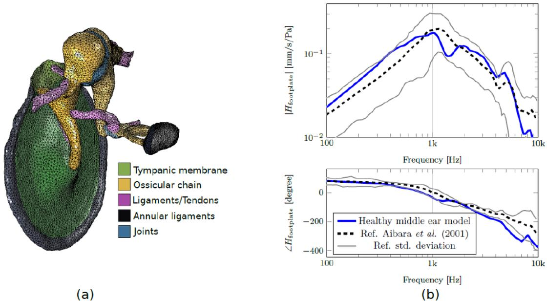
Figura 2: (a) FE model of the human middle ear and (b) numerical  $H_{\text{footplate}}$  compared to experimental data.
