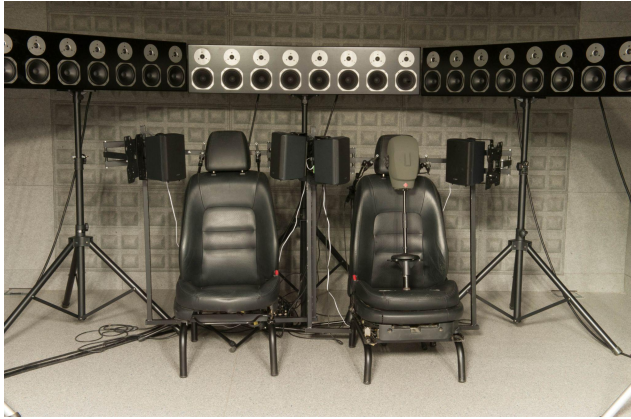
Figure 1. Car seats surrounded by sound transducers and microphones.
