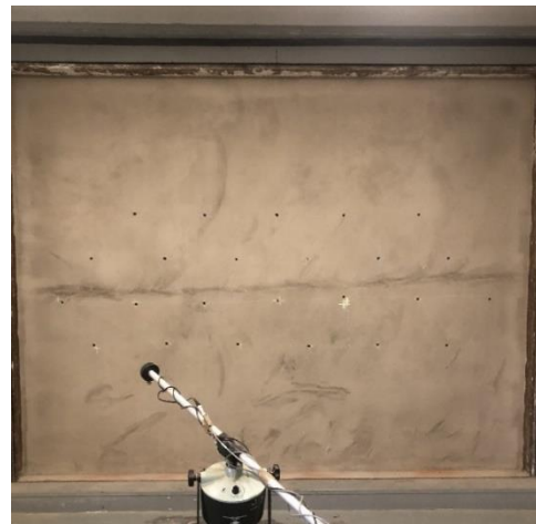
Figure 2. The 24 drilled holes for PHASE 1 measurements
