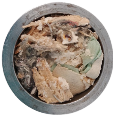
Figure 1. Mycelium composite from textile strips and sugarcane bagasse.
