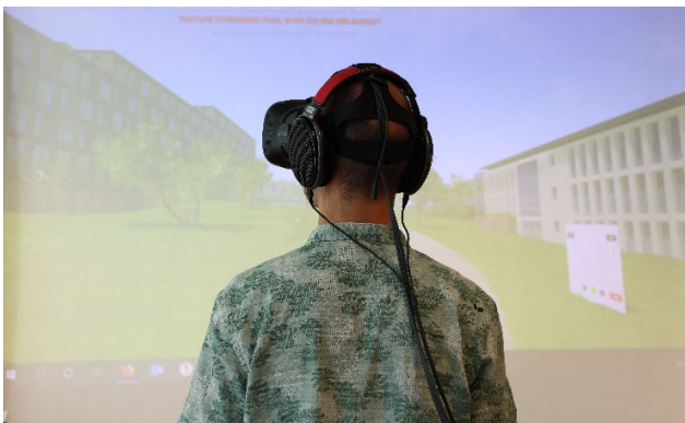
Figure 3 Virtual Soundwalk at the IHTApark using headphones and VR glasses. The participant is asked to make use of virtual GUIs to describe and rate the different scenarios.
