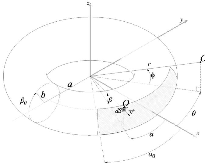
Figure 1 – Toroidal acoustic continuous source (gray). The torus is defined by its major radius  $a$  and minor radius  $b$ . The point  $Q$  is an elementary source of the active torus and  $O$  is an observation point.
