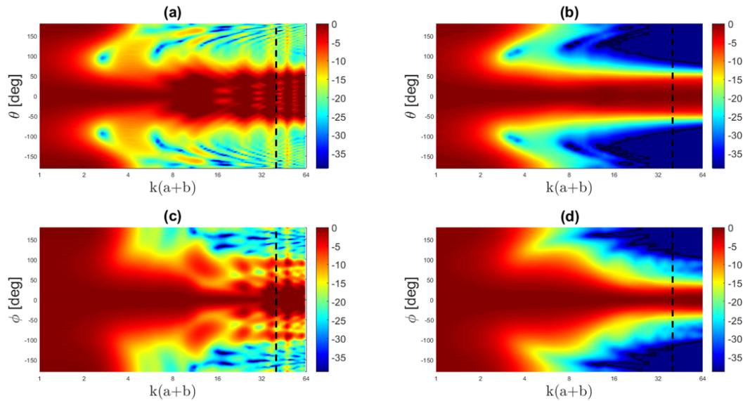
Figure 2 –Representation of torus directivity, with the a) HP with ES, b) HP with the 2DCS, c) VP with ES and d) VP with the 2DCS. For all cases:  $\alpha = 60^\circ$ ,  $\beta = 60^\circ$  and  $\sigma = 1$ .
