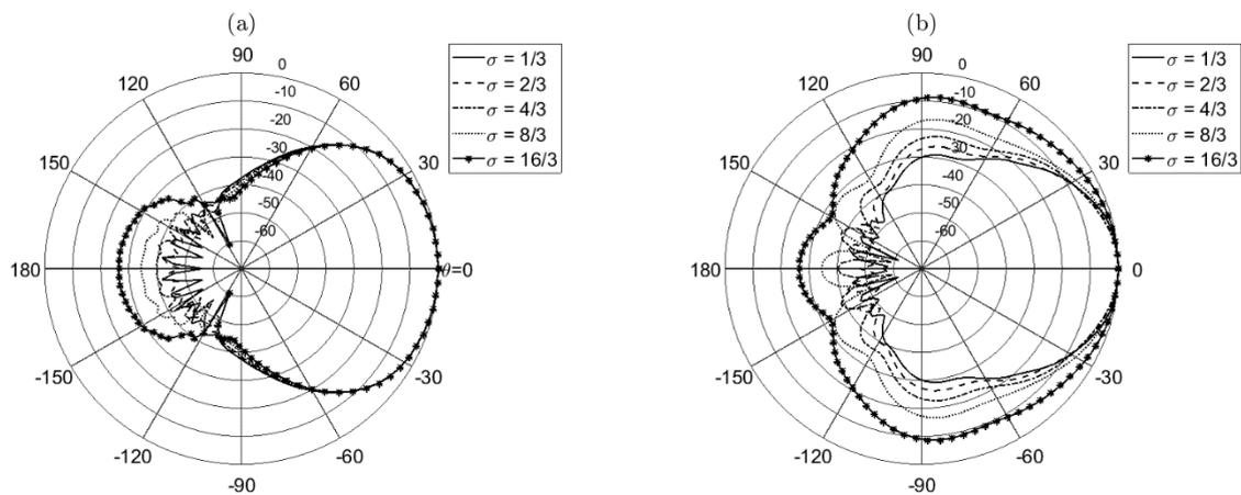
Figure 5 – Directivity pattern of the toroidal cap with 2DCS with  $\alpha_0 = 60^\circ$ ;  $\beta_0 = 40^\circ$ ;  $k \cdot (a + b) = 30$  in the a) HP and b) VP
