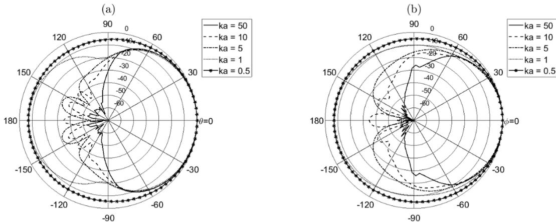
Figure 4 – Directivity pattern of the toroidal cap with 2DCS with  $\alpha_0 = 90^\circ$ ;  $\beta_0 = 90^\circ$ ;  $\sigma = 1.15$  with respect to the parameter  $k \cdot a$ , in the a) HP and b) VP.
