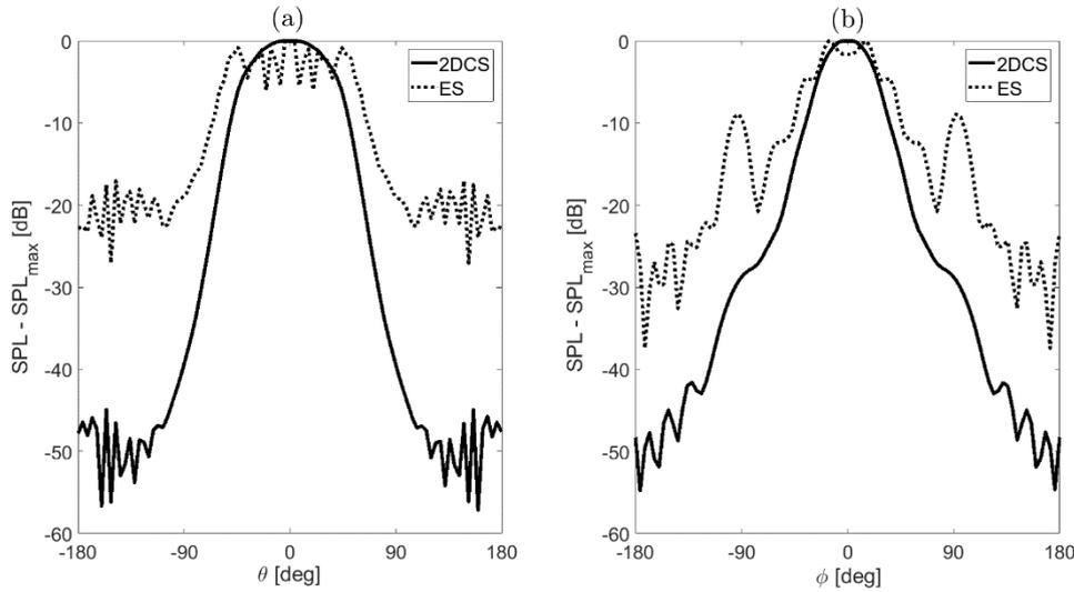
Figure 3 – Normalized Sound Pressure Level of the toroidal cap with 2DCS and ES at  $k \cdot (a+b) = 40$  in the a) HP and b) VP
