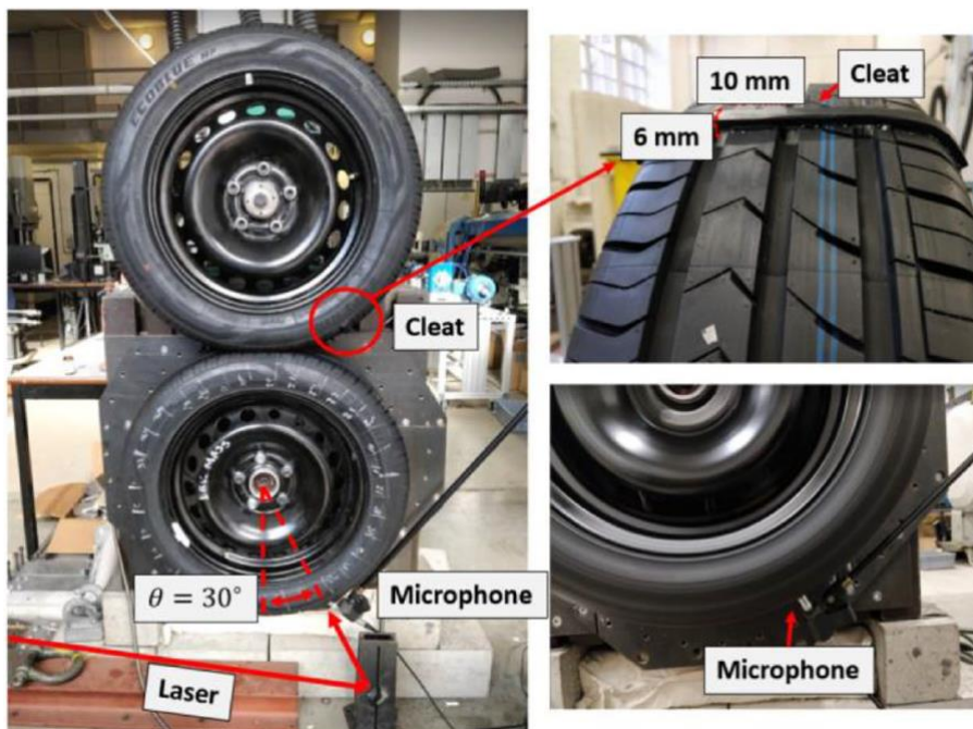
Figure 4: Illustration of the “tyre-on-tyre” setup for testing the tyre in rolling conditions [9].
