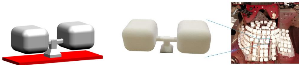
Figure 2: Illustration of the resonant addition on a UC (left) realized resonator (center) and the resonant metamaterial patch installed to the right shock tower in the vehicle (right).
