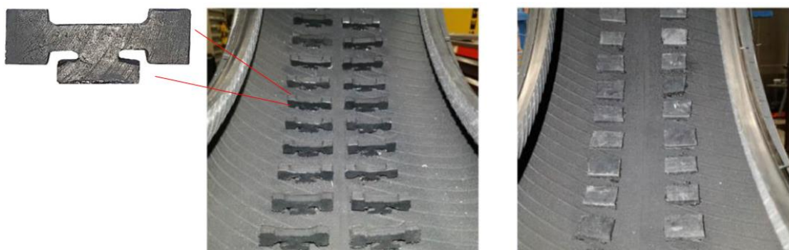
Figure 5: Illustration of locally resonant metamaterial tyre (left) and equivalent mass tyre (right) configurations [9].
