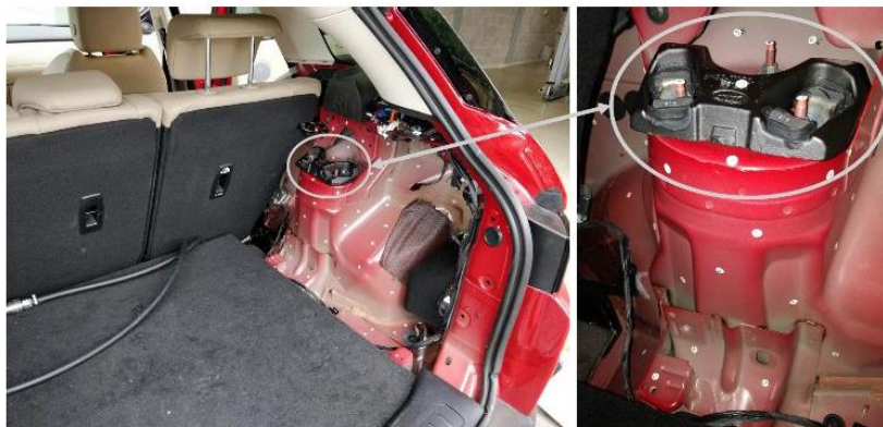
Figure 1: Illustration of the right rear shock tower of the vehicle with an installed TVA [7].
