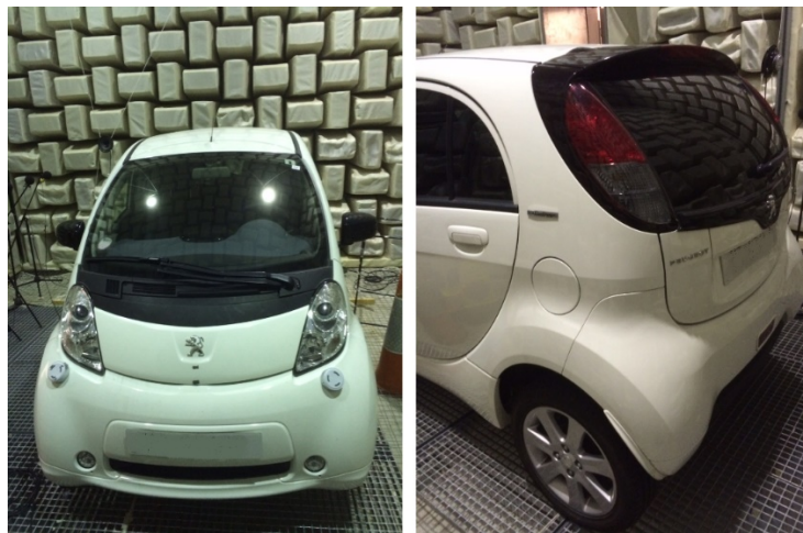
Figure 3: Vehicle inside the semi-anechoic chamber
