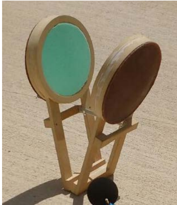
Figure 1: Clapper used as impulsive Noise source
