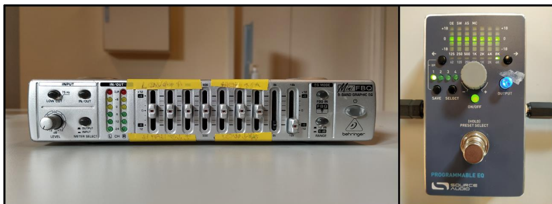
Figure 2 - Tested analog equalizers: Behringer MiniFBQ FBQ-800 (left, original equalizer); SourceAudio PEQ SA170 (right, tentative analog alternative).
