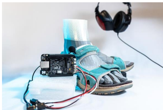
Figure 3 - Complete test system with the Bela.io implementation.
