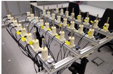
Figure 5. Grid of 4x8 Bruël & Kjær microphones Type 4958.
