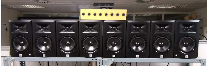
Figure 4. Picture showing the array of woofers, the array of tweeters and the 3D camera.
